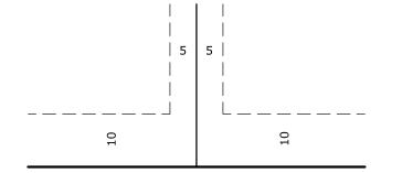
BEING 10 FEET IN WIDTH TO RIGHT OF WAY LINES, AND 5 FEET IN WIDTH TO ADJOINING LOT LINES UNLESS OTHERWISE SHOWN ON THIS PLAT.
